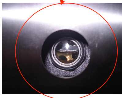
Figure 1. Rear display for checking the oil level
