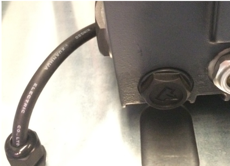
Figure 5. Remove the oil drainage plug
