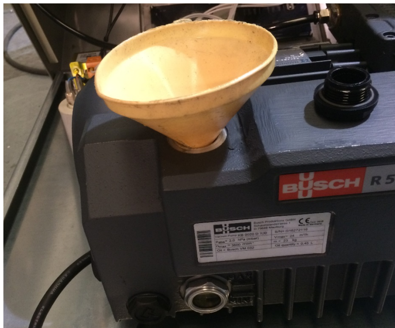
Figure 7. Remove the oil filling plug and refill with new oil
