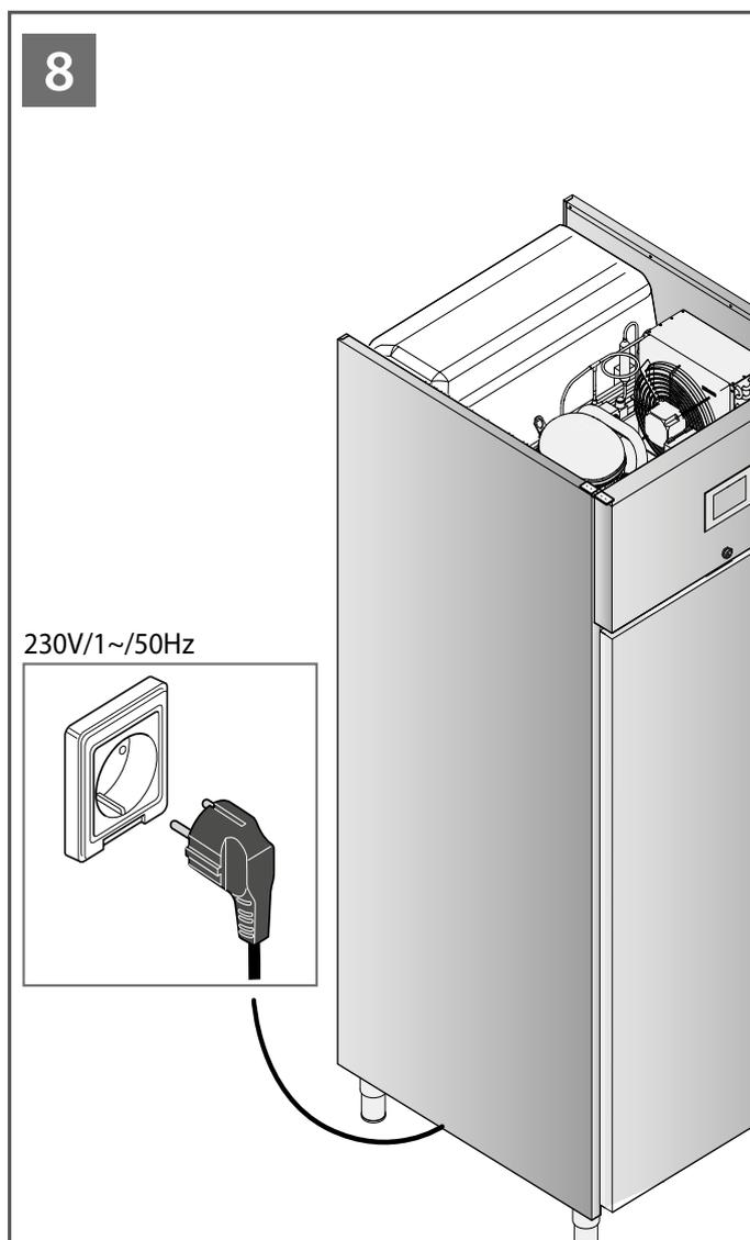
SYSTEM COMPLIANT TO THE LEGAL PROVISIONS IN FORCE (YELLOW GREEN CONDUCTOR WITH A MAXIMUM SECTION OF 10 MMQ - CEI EN 60335-2-42:2003-09 NORM). THIS CONNECTION MUST BE MADE BETWEEN THE VARIOUS DEVICES WITH THE TERMINAL MARKED WITH THE EQUIPOTENTIAL SYMBOL
