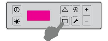
This function is active only if the device is in ON. When you press the button, you can immediately access the selection menu of the set point list of the two drawers. The sequence of the various phases is given below:
