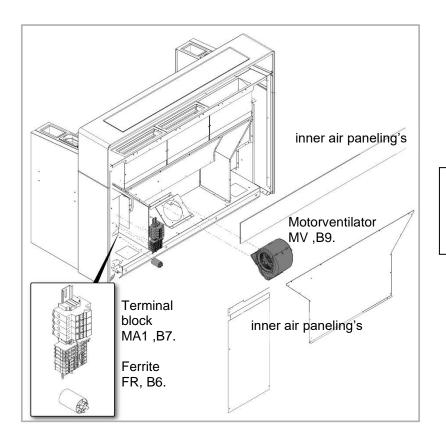
Once that the aesthetic panels have been removed, loosen the inner air paneling's to gain access to the rear components.
