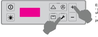
Exit from the MENU can be obtained: - pressing the SERVICE and UP keys simultaneously while a label is displayed - waiting TIME-OUT(90 seconds) without pressing any key..
