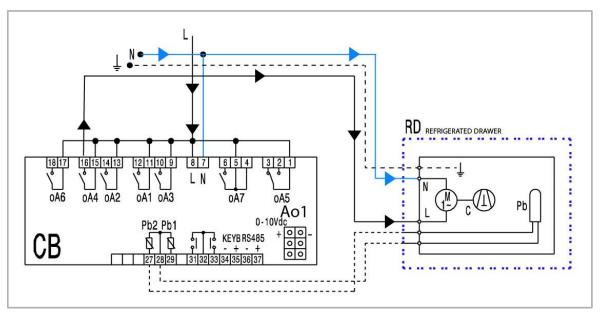
**Pb2 & Pb1** are analog inputs for PTC or NTC probes (10K at 25°C) configurable by parameter **P1C** and **P2C** see also <u>§PARAMETERS</u> <u>§DRAWER LEVEL SET</u>
