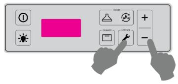
Pressing the SERVICE+DOWN keys for 3 seconds enters the parameters. The label of the first visible parameter appears. It is possible to scroll through the parameter labels with UP and DOWN. Enter into the value of each parameter value
