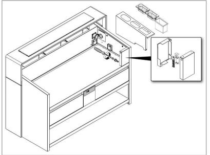
The sensor is located in the side panel. To gain access remove the back cover panel indicated in the detailed picture.
