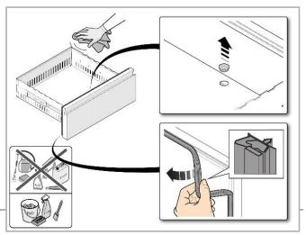
The **Gasket** is locked in place into a slot; it's a "press in" model, so it can be removed for a better cleaning.
