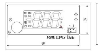
The Display is part of the U.I , it communicates to the membrane board, refer also to the §  $\underline{\text{B3,}}$   $\underline{\text{U.I.}}$
