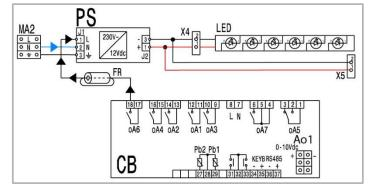
The function of the light button depends on the LPC (Light Push Configuration) parameter. If LPC = NU, the button is not used If LPC = LiG, the button on the U.I. is used to activate the light output. When the light button is pressed on the U.I, the relay output of CB is oA6. The Light button is active both in OFF and in keyboard lock. One or two Led Bars (contact X4 & X5) are supplied 12V from the PS voltage adaptor.
