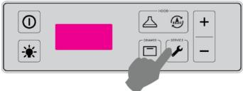
**PROCEDURE:** When you press the service button , you can immediately access the menu; the display shows the first label "dP1" and the "° C" or "° F" icon starts flashing to indicate access to the MENU. By pressing the SERVICE key, the value of the selected variable is displayed. Press "SERVICE" to view the next label. With UP and DOWN you can quickly scroll through the list of menu items.
