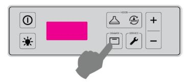
This function is active only if the device is in ON. When you press the button, you can immediately access the selection menu of the set point list of the two drawers. The sequence of the various phases is given below:
