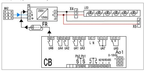
The Ferrite "FR" bead is a passive device that filters high frequency noise energy over a broad frequency range. It becomes resistive over its intended frequency range and dissipates the noise energy in the form of heat.
