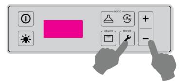
Pressing the SERVICE+DOWN keys for 3 seconds enters the parameters.
