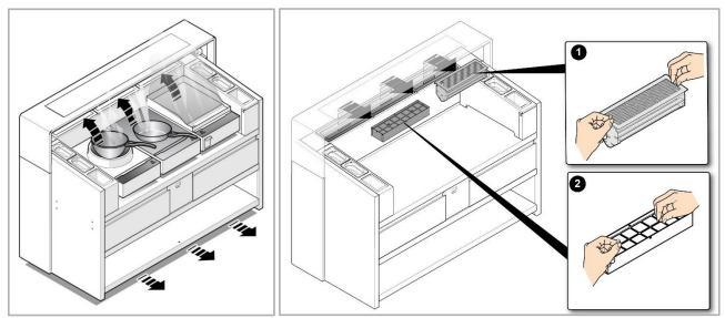
Filter cleaning refer to § FILTERS (GREASE & CARBON).
