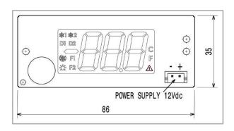
The Display is part of the U.I , it communicates to the membrane board, refer also to the §  $\underline{\text{B3}}$ , U.I.
