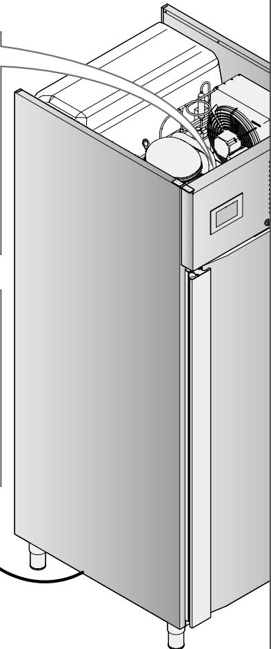
SYSTEM COMPLIANT TO THE LEGAL PROVISIONS IN FORCE (YELLOW GREEN CONDUCTOR WITH A MAXIMUM SECTION OF 10 MMQ - CEI EN 60335-2-42:2003-09 NORM). THIS CONNECTION MUST BE MADE BETWEEN THE VARIOUS DEVICES WITH THE TERMINAL MARKED WITH THE EQUIPOTENTIAL SYMBOL
