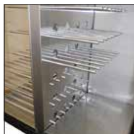
A2. Move towards left 3 rows of rods or unscrew them (Depends on the model)
