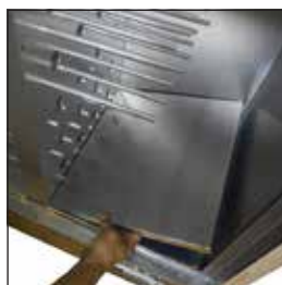
A3. Remove the aluminium panel
