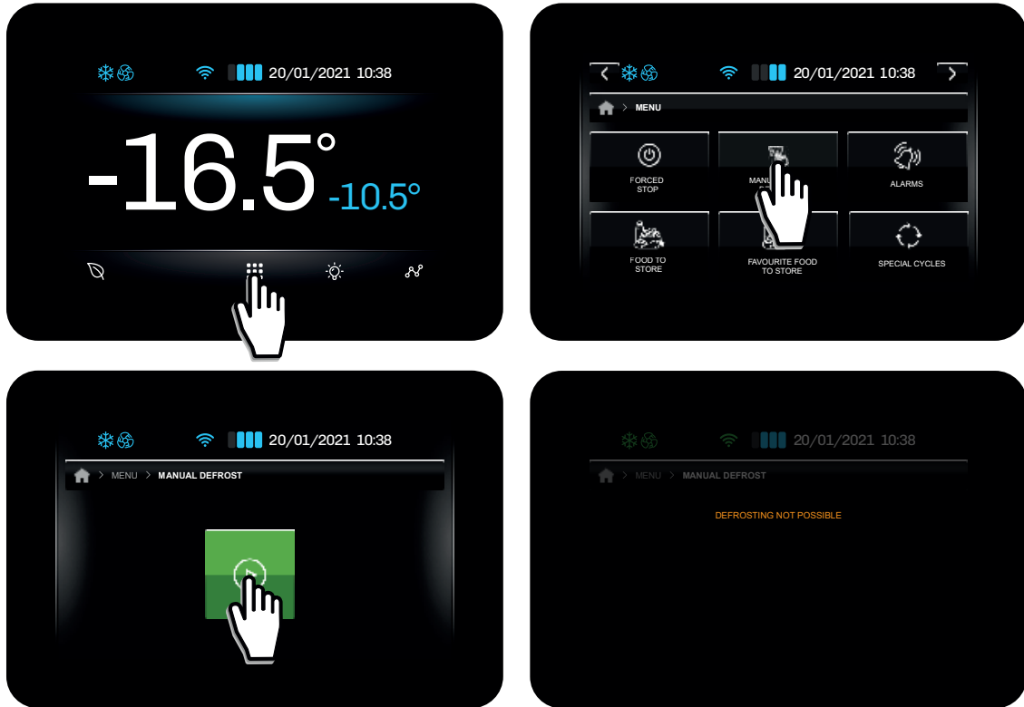
Manual defrost not possible
