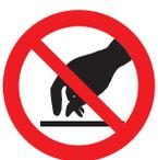
This symbol identifies the prohibition to carry out work on live systems, to touch systems unless authorized, to remove the guards and safety enclosures before having disconnected the voltage.
